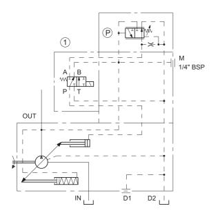
The PCM pressure regulator allows, by means of a suitable solenoid valve, the electrical switching of the pump displacement from the maximum to the minimum (or zero) value.
