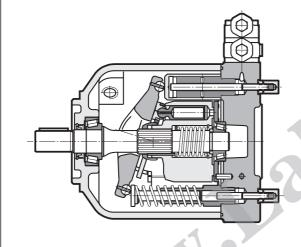
constant and 350 bar peak). Thanks to some particular design features, these pumps are able to bear high axial and radial loads on the shaft.
