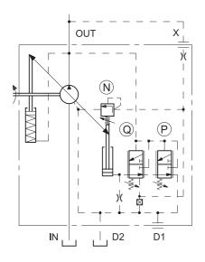
Such regulator keeps the pump torque at a constant level by changing the displacement according to the delivery pressure, so that the ratio  $p \ge Q$  (absorbed power) remains unchanged. The functions limiting the (P) maximum pressure and regulating the (Q) flow rate are always present, if a restrictor has been installed on the user line.
