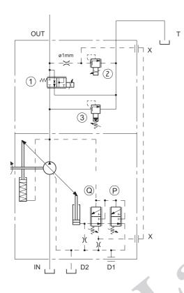
This regulator allows an independent regulation of the pump flow and pressure, both with an electric proportional control.
