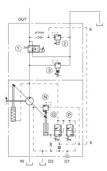
This system combines all the functions of the constant power control as a standard PQNC regulator, and moreover it allows the independent proportional regulation of the pump flow and pressure at values behind the power curve characteristic set on the regulator  $\widehat{\mathbb{N}}$ .
