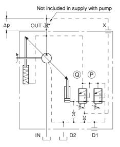
This regulator, apart from regulating the pressure (as for the PC model), allows the pump flow rate to be regulated according to the  $\Delta p$  pressure drop measured on either side of a throttle valve installed on the user line. The connection pipe between the X port and the flowline downstream the restrictor (or valve) must always be made (customer charge).
