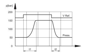
The response times are obtained with a VPPM-046 pump, by changing the reference signal (V Ref)on the proportional valve in order to have a line pressure variation from 50 to 150 bar and vice versa, with an oil volume of 5lt.
