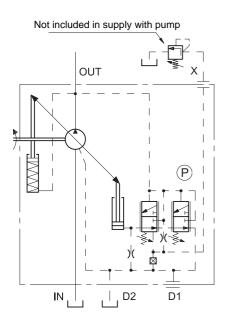
The PCR regulator, apart from limiting the line maximum pressure (Pvalve), allows a remote-control of the device via a remote control connected to the X port (typical application for submerged pumps). In case a pressure regulating valve is used for the remote-control, it is suggested to use a direct operated valve with a size suitable to 1,5 l/min pilot flow rate.
