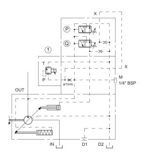
The PCX regulator mated with a proportional pressure relief valve, allows a continuous control and modulation of the system pressure.
