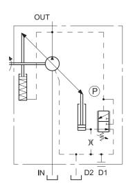
The PC pressure regulator keeps the pressure at a constant set level in the circuit, thus adjusting automatically the pump flow rate according to the real need of the system.
